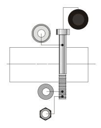
Figure 7. Configuration for 6" bolts.
